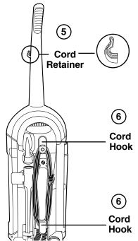
5. You will find your cord retainer on the handle above the upper cord hook. Firmly push the electrical cord down into the cord retainer. This will place the cord out of the way the next time you vacuum.
